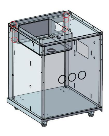
Before proceeding to the next Installation Guide, ensure you've correctly assembled the Flare Free cup from the Coleman Revolution BBQ package. Fit it snugly into the module front panel cutout.
