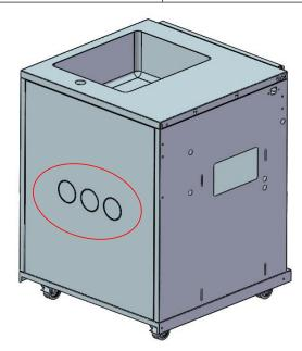
Identify and open the appropriate cutout that suits your kitchen's requirements, like drainage or cold/hot water supply.
