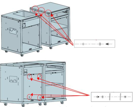
Insert the fastening clips from the bottom upwards, applying some force. This may require a bit of effort, but it ensures the units are securely connected as intended.
