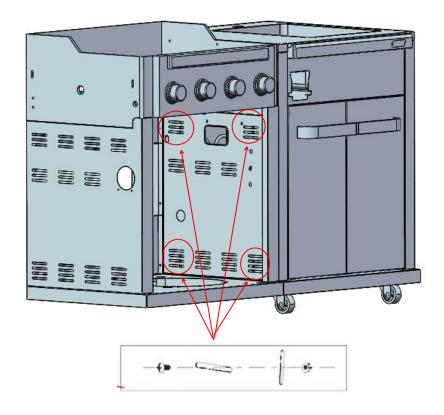
Insert the fastening clips from the bottom upwards, applying some force. This may require a bit of effort, but it ensures the units are securely connected as intended.
