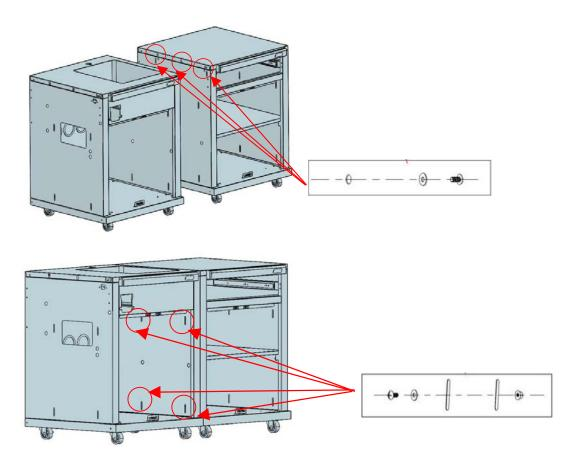
Insert the fastening clips from the bottom upwards, applying some force. This may require a bit of effort, but it ensures the units are securely connected as intended.
