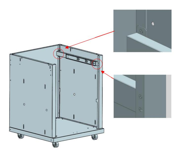
Install both the left and right rails following the same procedure.
