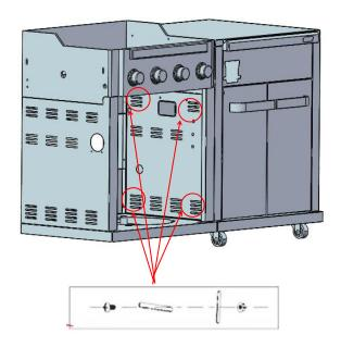
Insert the fastening clips from the bottom upwards, applying some force. This may require a bit of effort, but it ensures the units are securely connected as intended.
