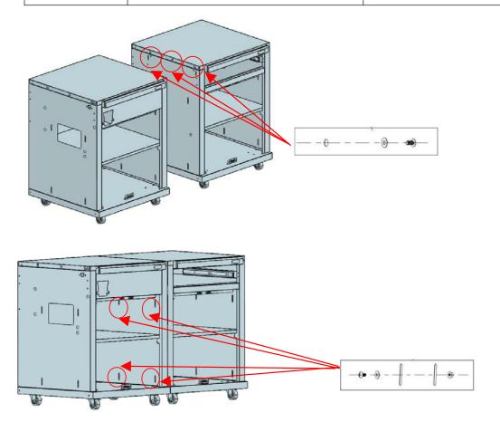
Insert the fastening clips from the bottom upwards, applying some force. This may require a bit of effort, but it ensures the units are securely connected as intended.
